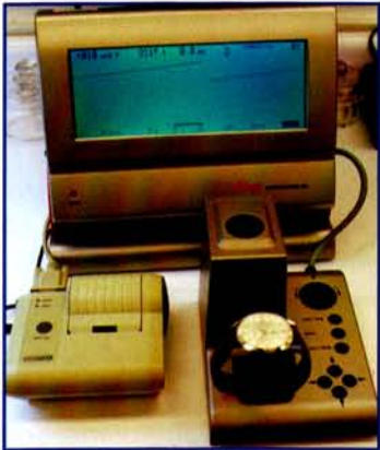
Equipment to measure the accuracy, amplitude and beat of mechanical watches.
